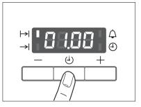
Using the function End time →, set the time at which the dish is to be ready. In this example, 14:05.
